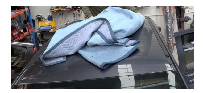
76. Place a soft blanket over the roof to protect it while lifting the roof rack on.
