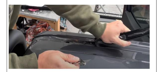
66. Using side cutters or a box cutter trim the rubber trim at the marked location.
