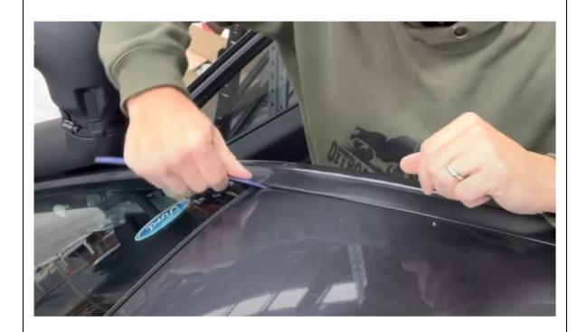
72. Move to the front of the car and using plastic trim tool remove the front edge of the rubber trim up to the stud again like the rear.
