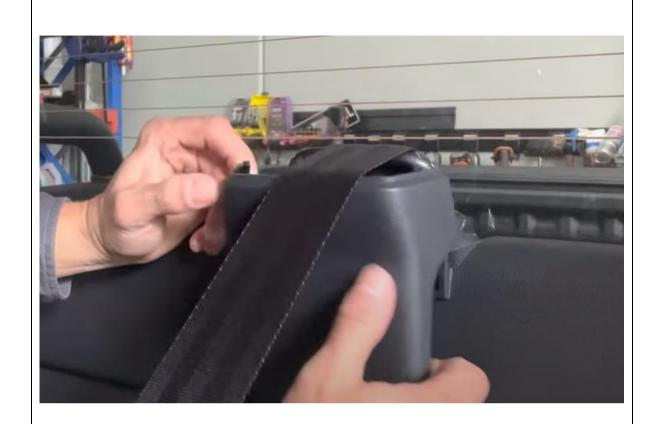
51. Peel and unclip centre seat belt cover by pulling top away from the rear bulkhead.
