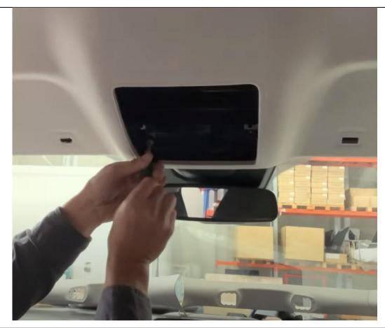
32. Using a T20 torx bit remove 2 screws shown.
