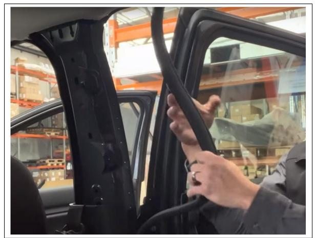
44. Peel rubber seal from sides and top of each 4 doors.
