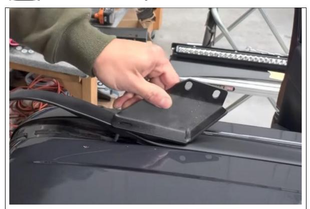
64. Place rear bracket on roof as shown and line up rear stud with centre of mounting slot.
