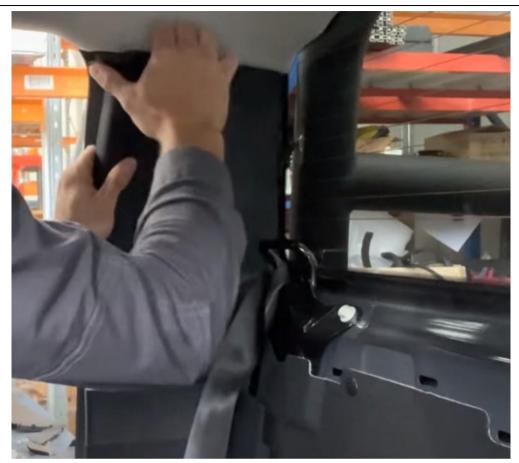
54. Remove the outside upper trim panel by pulling from the top and working your way down.
