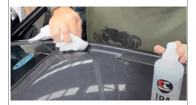
77. Using a cleaning solvent like isopropyl alcohol gives all the exposed ditch areas a good clean.
